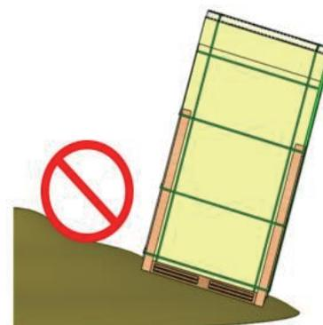
Inclined slopes of  $>4^\circ$
