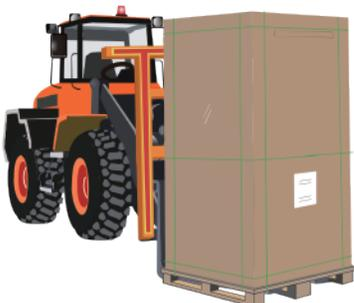
Unloading long-side vertical package by forklift
