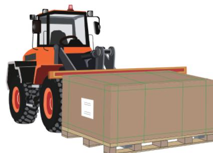
Unloading short-side vertical package by forklift
